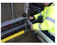
Fit both Legs using the Pins and 'R' Clips provided and ensure that the Pins are inserted outside in, to minimise the risk of the 'R' Clips being Knocked out. *REMEMBER:* Fit the Legs to the '**Normal use'** hole Labelled on the underside of the platform.
