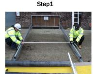
Lay out the components ready for assembly with the platform against the wall with wheels on the ground. Identify the corresponding Leg for each side of the platform (Green – Left / Red – Right)
